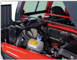
The **4-cylinder turbo diesel engine** of **emission stage 3B** is powerful and environmentally friendly at the same time. Equipped with a particle filter, it impresses with 70 hp, high pulling power, smooth running, and long service life.
