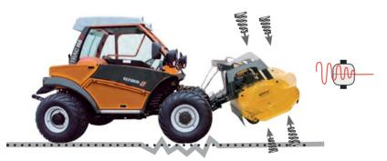
The impact load is minimised by gas pressure accumulators.
