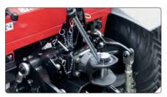
Mechanical or automatic **trailer hitches** are available for different applications.
