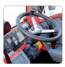
The **tilt-adjustable steering column** ensures an optimum seating position.
