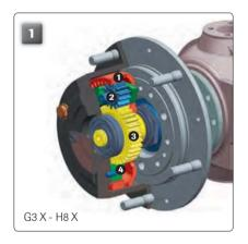
Robust driving/steering axles with **planet gear final drives** deliver high pulling force and protect the drive train. The drive shafts are exposed to lower forces, therefore they can be built in a lighter design.
