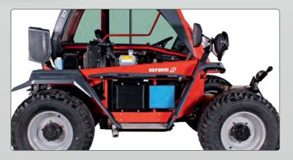
For the H7 RX, the emphasis is on **serviceability** and optimal accessibility of the components. All service and maintenance flaps can be opened easily and without tools. This particularly facilitates the daily service work such as checking and servicing of windscreen washer fluid, air filter, engine oil level, brake fluid reservoir, clutch fluid, etc.
