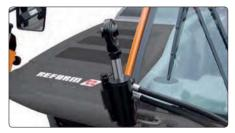
With the **hydraulic top link**, you can react to uneven ground quickly from the cab or adjust the working depth with the push of a button.
