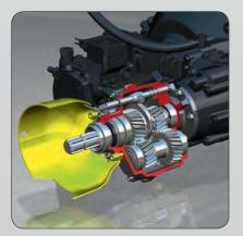
In order to satisfy individual customer requirements, two different speeds (540 and 1,000 rpm) can be selected on the H8 X both on the front PTO and at the rear PTO. This give you always the **appropriate PTO speed** for your attachment.
