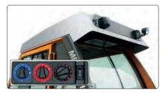
Comfortable climate with roof-integrated **air conditioning** or additional fresh air supply for closed cab with the integrated **roof ventilation system** (not with G7 RX / H7 RX).
