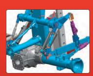
Extra Stability is achieved by supporting the rear linkage with pull rods on the rear axle.
