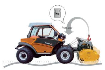
The tool follows the ground contours without changing the weight compensation pressure.
