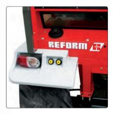
The easily accessible **filler neck** provides for fast filling stops, and the **electrical external control** for the linkage makes mounting and removing of attachments easy.
